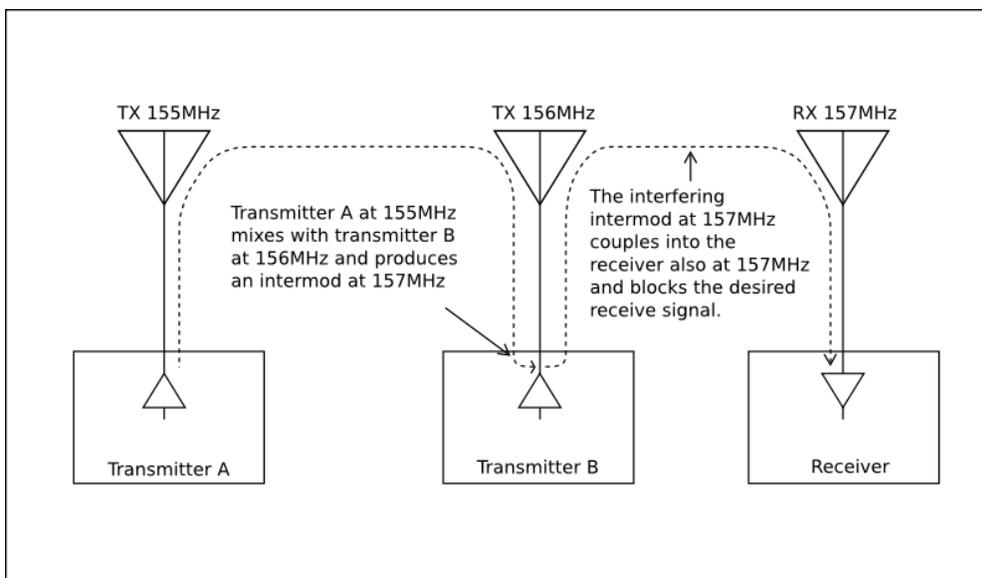
Figure 2 – Intermod generation at a communication site
