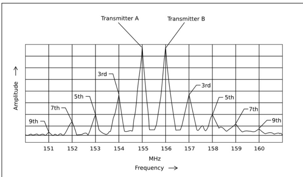
Figure 1 – Intermodulation products created due to transmitter mixing
