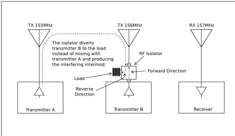
Figure 3 – RF isolator prevents mixing of transmitters
